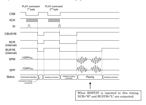
NCR outputs "L" during command processing and address administration, and outputs "H" in other state. BUSYB outputs "L" during command processing and reproduction, and outputs "H" in other state. NCR/BUSYB at the time of inputting the RDSTAT command is read as the serial output from SO terminal.
