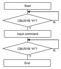
2-Byte Command Input Flow (applied to the AMODE, PLAY, FADR, MUON, CVOL, AVOL, VPITCH, and VSPD commands)
