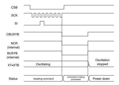
The speaker amplifier stops operation after a lapse of command processing time after the PDWN command is input. At this time, the SPM output of the speaker amplifier goes to "Hi-Z" state to prevent troubles by pop noise.
