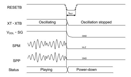
Note: The same timing is applied in the case that the RESETB signal is input during command waiting.
