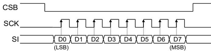
◆ Input timing when 2-byte command is selected
