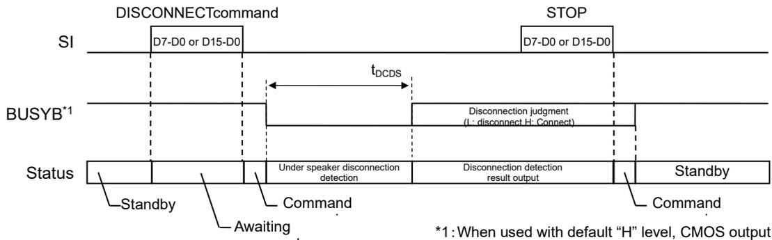
When no STOP command is input after the execution of DISCONNECT command, the disconnection detection automatically stops in one second, and transition to standby occurs.
