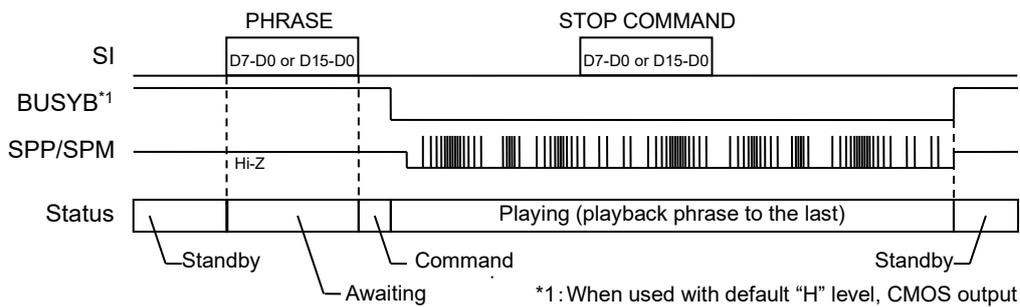
◆ STOP command operation in the case of Change Immediately Once mode or Change Immediately mode
