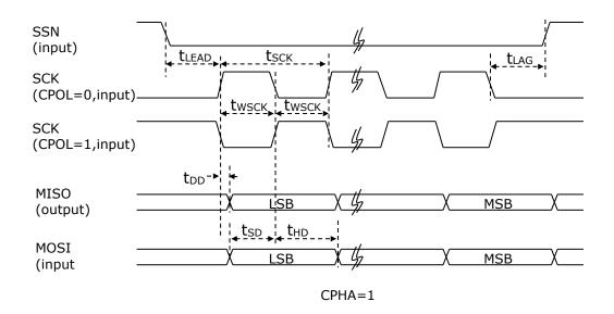
$\ast$  CPHA and CPOL registers set the data output timing and clock polarity.
