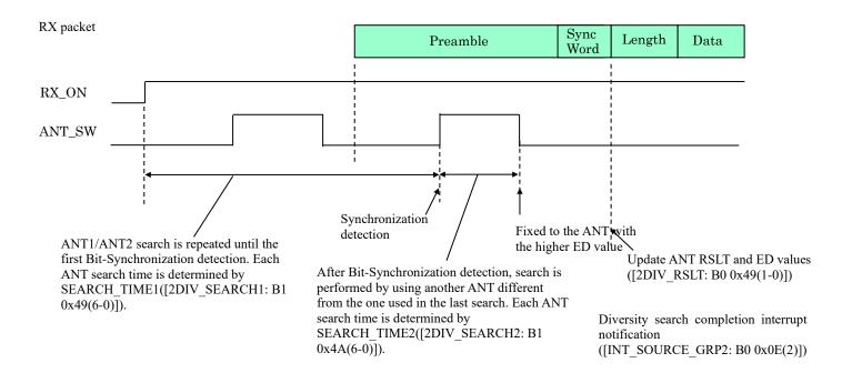
ED value obtained by Diversity ([ANT1\_ED: B0 0x4A]) or [ANT2\_ED: B0 0x4B]) and Diversity antenna result ([2DIV\_RSLT: B0 0x49(1-0)]) are updated and overwritten when SyncWord is detected. The number of detection performed during the ED value calculation is specified by 2DIV\_ED\_AVG([2DIV\_MODE: B1 0x48(2:0)]). Time resolution of search times ([SEARCH\_TIME1] and [SEARCH\_TIME2]) can be specified by SEARCH\_TIME\_SET([2DIV\_SEARCH1: B1 0x49(7)]).
