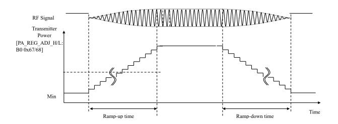
In the reset state and the maximum value setting (FREF = 48MHz, PA output power + 13 dBm), the example of ramp-up and -down times will be as follows:
