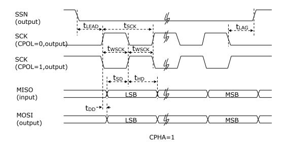
\* CPHA and CPOL registers set the data output timing and clock polarity.
