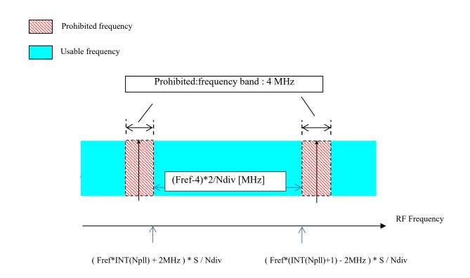
(2) CH#0 frequency and channel interval settings may have error. Therefore, channel frequency has frequency error indicated by the following formula.
