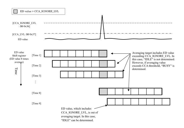
The following is the timing diagram when ED value under strong signal input was acquired.
