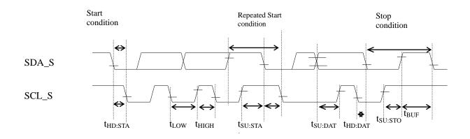
If powering off ISO\_V of this LSI, it disables communications of other devices on the I²C bus. Even when there is no receiving power from the P\_ANT pin, the SDA\_S/SCL\_S pin will maintain the Hi-Z state when there is a power input on the ISO\_V pin of this LSI.
