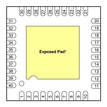
\*Solder the exposed pad onto the PCB
