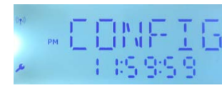
Figure 7 Display of the LCD after clicking the <Reset and Restart> button of the DTU8 debugger
