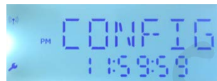
Figure 12 Display of the LCD after clicking the <Reset and Restart> button of the DTU8 debugger
