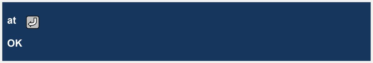
Fig. 3-2 : Result code string output screen for command reception confirmation
