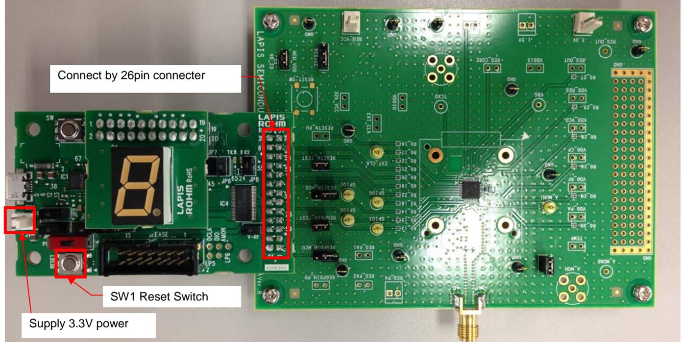
Figure 2: ML7344 Evaluation Board Connection Overview
